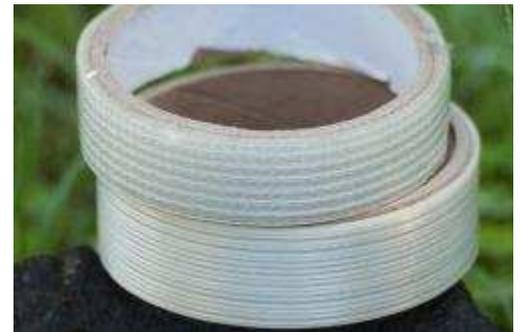
Particularly if you are using the straight-laid version of this tape, your fuselage will be stronger if you wind the tape in a spiral pattern around the rear of your fuselage (start from the tail-end and work forward for best results). I don't think the extra weight is something to be concerned about, as in my opinion, stock Radians tend to be slightly nose-heavy, so adding a little weight to the rear-end may help improve performance (and would meet Mr. Charles' approval, I'm sure).
