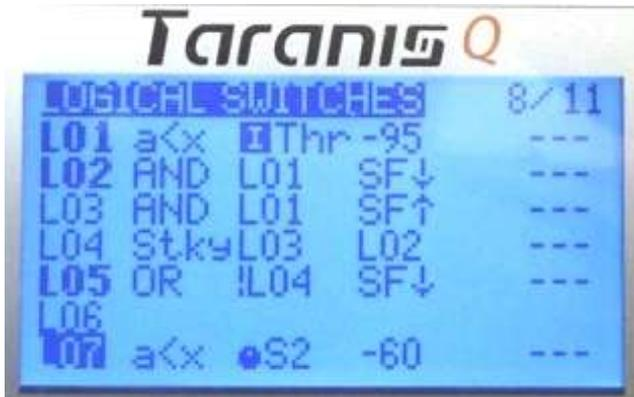
On the left we see that L02 is now ON, which both turns off L04 (motor armed) and turns on L05. Remember L05; it is the switch that activates the special function to cut the throttle.
