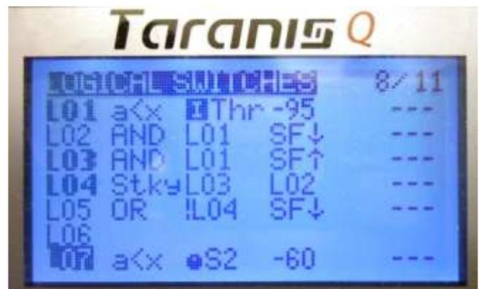
The bold characters show which logic switches are “on” so L01, L03 and L04 are all on which means that the throttle will function; L04 has in fact been turned on by L03. It will be turned off when I throw switch SF into the throttle cut position which will activate L02.
