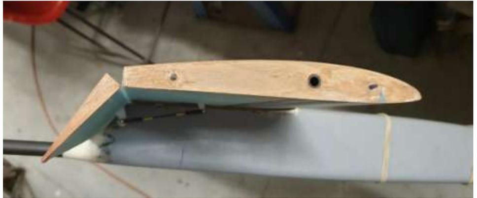
surface to make a live hinge for the centre flap – I forgot and used tape later. As this was meant to be a simple, speedy, build (ha!). I just rolled on epoxy laminating resin and made no effort to scrape off the excess. The end result was a bit heavier than I expected, but was very stiff – I could not flex it very much at all.
