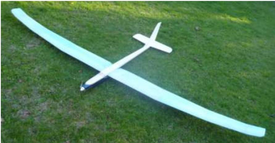
Weight 1.67 kg 3.2 meter wing span.
