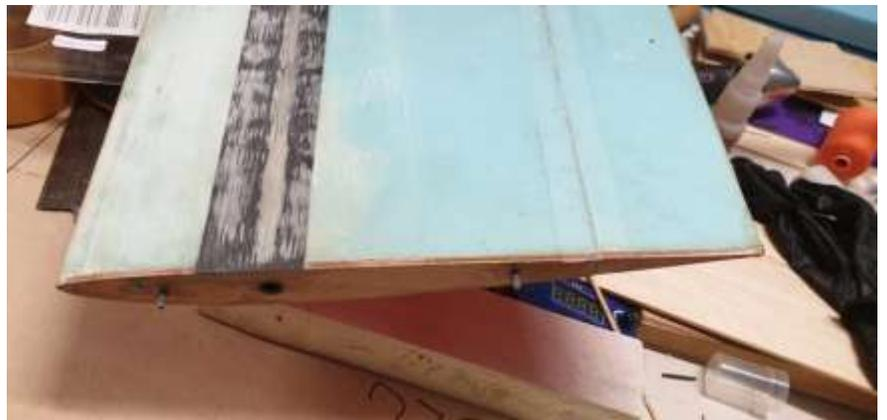
the core/skins. The ply rib also reduced the potential for the carbon tube to split from the load of the 6mm piano-wire wing brace, which is inside the tube. Some 50mm wide, 80GSM uni-directional carbon fibre was added top and bottom of the core for bending stiffness and 55gsm glass was added on a 45/45 degree bias for torsional stiffness. All of the fibers overlapped the ply ribs, with the excess cut off when the resin had cured. No Kevlar was added along the bottom
