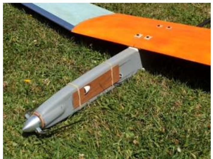
The access hatch is simply some 1.2mm plywood held in place with two rubber bands at the moment. I did add a small plastic scoop to get some air in to cool the ESC – this has worked well. With everything in place the CoG was a little off and a heavier spinner was used.
