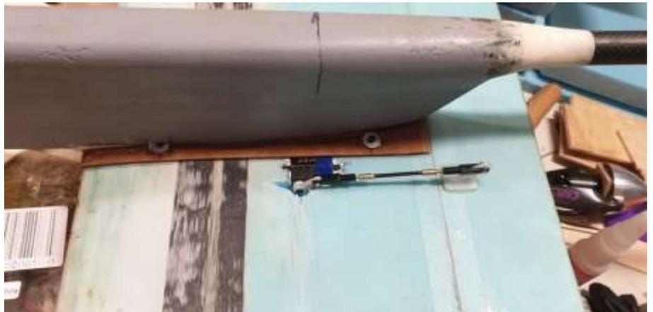
These have two purposes: the first is that the wing-saddle mount is glued and screwed directly to these ensuring a stiff connection between the wing and the fuselage. The second function is to provide a stiff connection between the carbon
