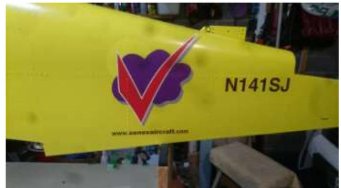
My model has lots of scale mushroom rivets and I found that I could press down quite hard with a swab of toilet paper on each rivet to shape the decal paper over the rivet to give that painted on look. Leave the decals to dry overnight, remove the masking tape and finish with 3 or 4 coats of clear to provide physical and UV protection. On my model I used automotive acrylic clear to finish the model's surface.
