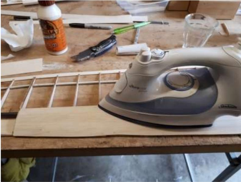
Set a clothes iron on wool with steam open. Fold the sheet down once more. Use the steam iron to wipe across each rib from back towards the LE. Move along to the next set of ribs. When cool, the job is done!
