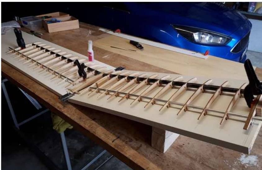
Assemble all ribs onto the spar. Have ribs #2 clamped to their blocks. The end ribs (3 laminated) must be now attached to the spar at exactly 90 deg. and flush with the end. When in place glue the build tab to the board then the rib to the spar. Now locate each rib progressively making sure tabs sit on the board and the rib is at 90 deg. Use the rib gluing jig shown on the plan. Tack in place with thin CA. Slide in the aluminium tubes and tack in place with thin CA.
