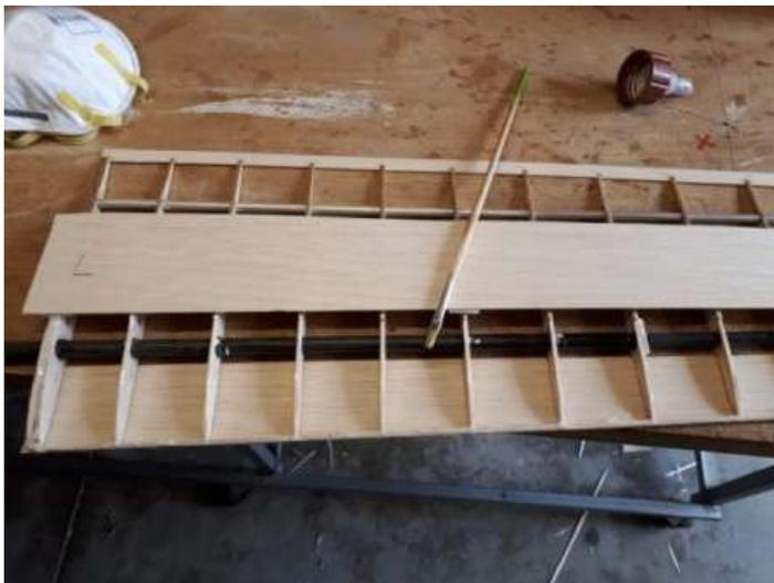
Fold the sheet back. Apply PVA glue to the edge of the ribs. Fold down the sheeting and gently rub on top of each rib.
