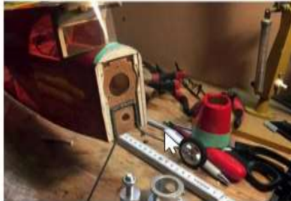
The 45 year old Tom Boy with the engine and 27MHz RC gear removed ready for a small brushless motor and 2S Lipo battery to be installed, along with modern FrSky RC gear.
