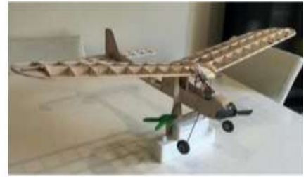
Ian Jemmeson's PAAGEboy for Indoor flying, C of G being checked before covering the model.
