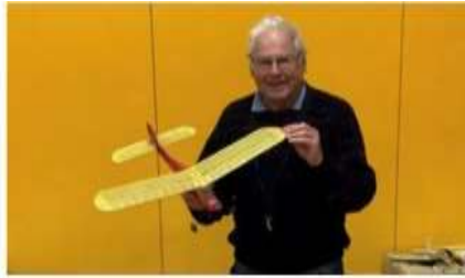
Ian Jemmeson's 60% size PAAGEboy for Indoor Flying, still flying well five years after it was built. It has a small 2s Lipo battery and Spectrum Rx on 2.4G driving a small brushless motor.
